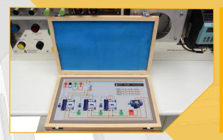
Static Automation modules are provided to expose users to actual industrial applications of PLC and HMI. These static automation modules represent various industrial processes which can be operated in integration with PLC and HMI. Banana connections are provided on static automation modules for PLC input and output connections. Depending on the user's requirement, various static modules are supplied along with PLC – HMI training kits.
