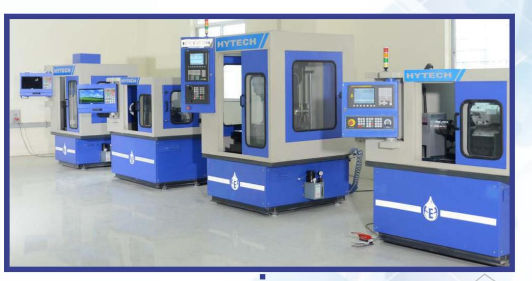
Once the program is successfully executed on NC Guide software, the same can be executed on Fanuc hardware simulator. Advantage of hardware simulator is that it gives an exact experience of Fanuc CNC controller so that students can get necessary confidence to operate the actual machine. Hardware simulator is equipped with Speed as well as Feed override along with all other functions available on Fanuc MOP. It is nothing but an actual Fanuc CNC without the machine.
